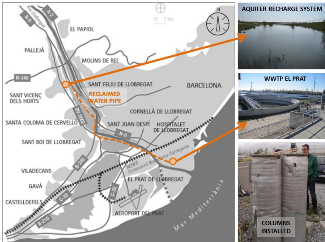
Figure 1: Location of the WWTP in El Prat del Llobregat and the MAR system in SVH NOTE: Dashed line represents the connexion pipe between the WRP in El Prat del Llobregat and the MAR system in Sant Vicenç dels Horts.
