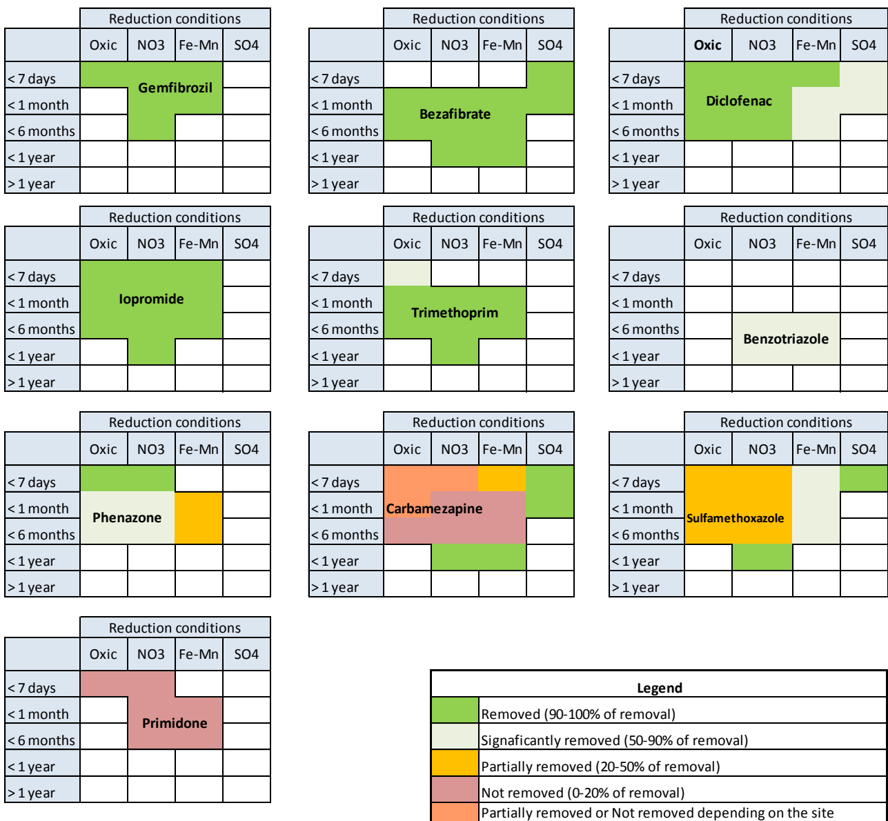
Figure 57: Matrix of the elimination of emerging pollutants in MAR systems Source: literature survey based on field experiences
